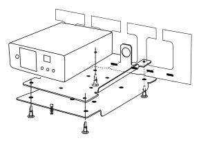
The HS-MOD001-BRKT supports the HS-VM1100 modulator for installation in a Concourse cabinet. This bracket comes complete with the small mounting plate required to complete the installation. Before installing the module, confirm that the package contains the following parts: one bracket, one mounting plate, one 5/16" hex nut and four plastic standoffs.
